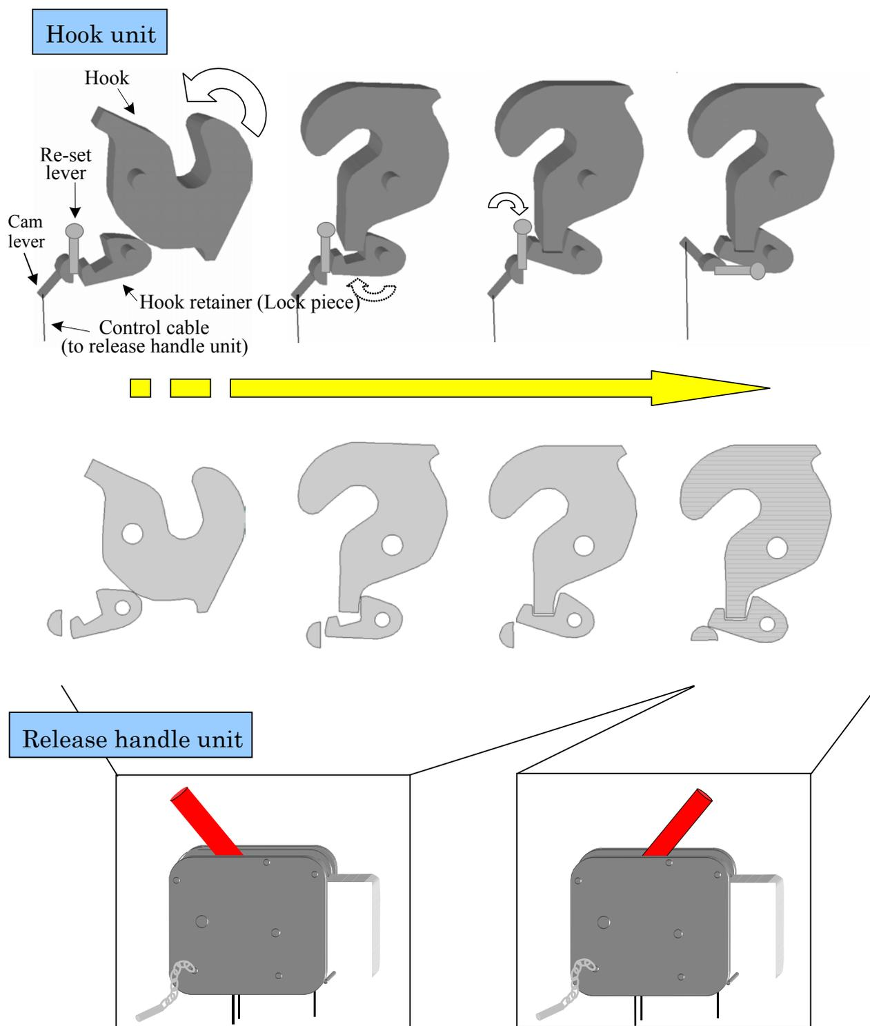
**Fig. 5.2.3 Reset principle of the hook unit**
