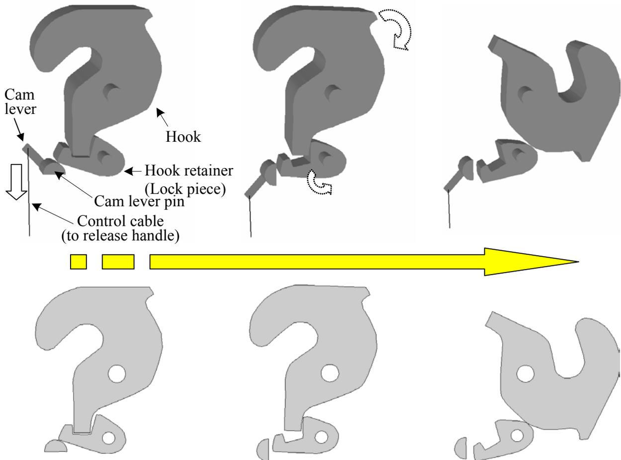
**Fig. 5.2.2 Release principle of the hook unit**
